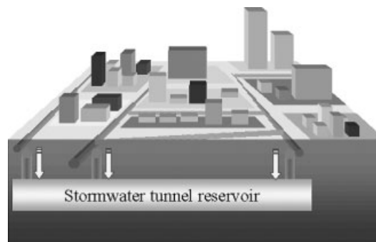
Figure 2. Diagram of flooding control system (II).
